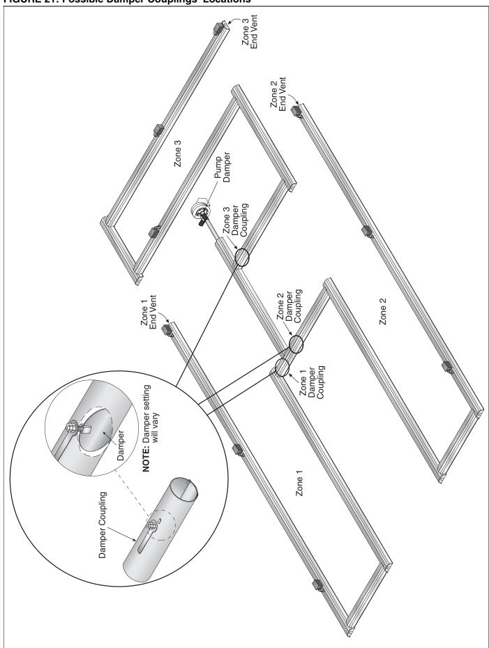
**Step 7.1.3** After setting end vent vacuums between 2.5" wc and 3.0" wc, while all the burners are still operating, use the down arrow button on the VFD to reduce the frequency of the output signal to the pump. Reduce the frequency of the VFD until the manometer at each of the end vents reads 1.0" wc - 1.2" wc Make note of this frequency setting below. The frequency is found on the VFD's LCD screen.
